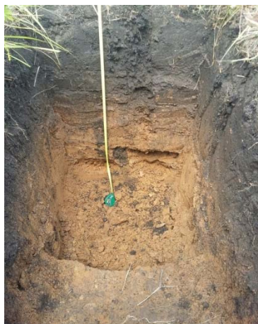
Figure 1. Leached medium-thick low-humus heavy loamy chernozem on mantle carbonate loams (arable land, coordinates: 51°931'094"; 9°293'506")
